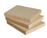
Manufacturing of PB, or chipboard, an engineered wood product manufactured from wood chips, sawmill shavings or sawdust, binded with synthetic resin
